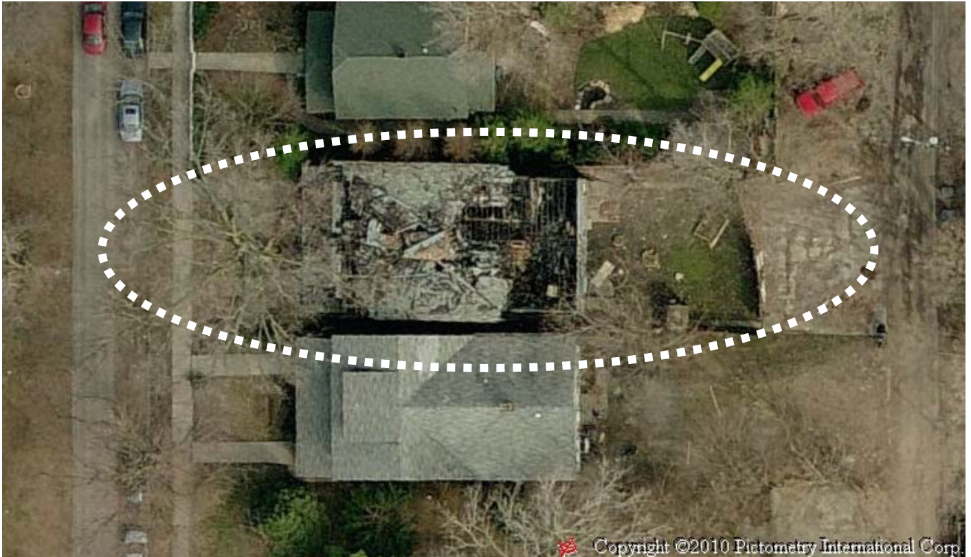
Aerial photo showing roof shortly after the fire, but prior to the remainder of the roof being removed as part of the emergency demolition.
