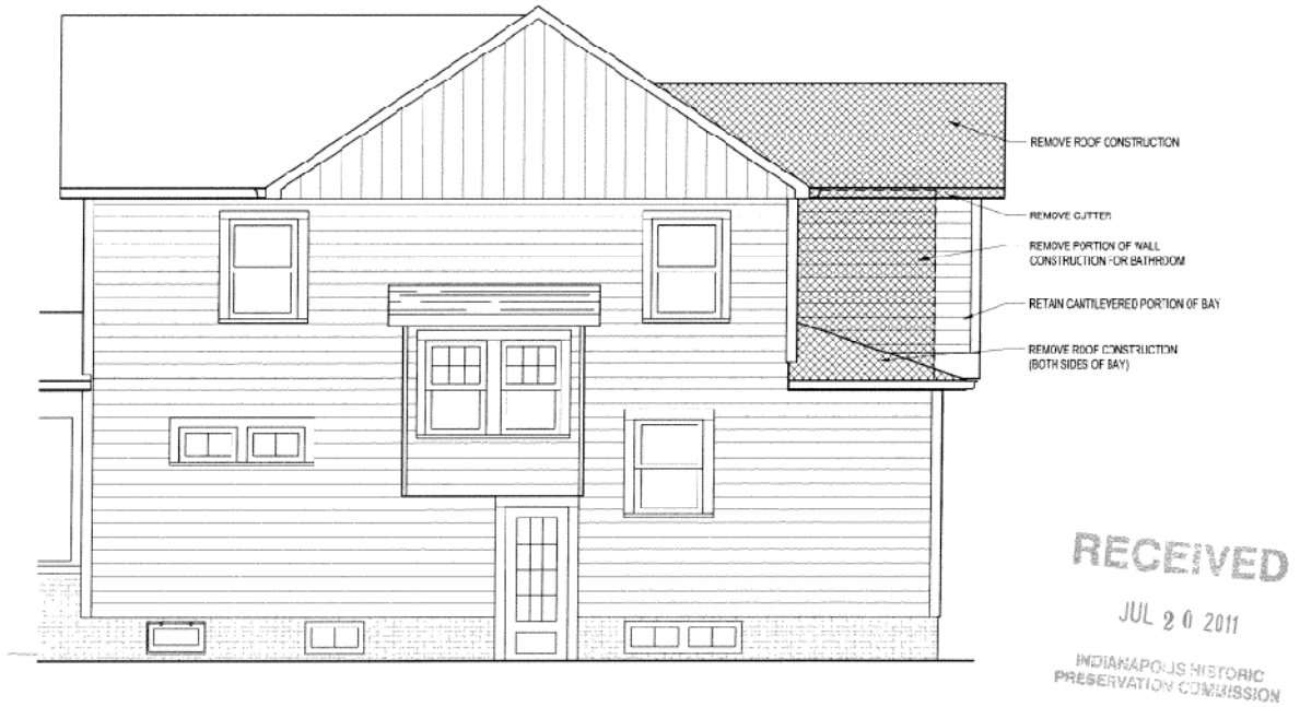
EXISTING NORTH (SIDE) ELEVATION SHT. D2
