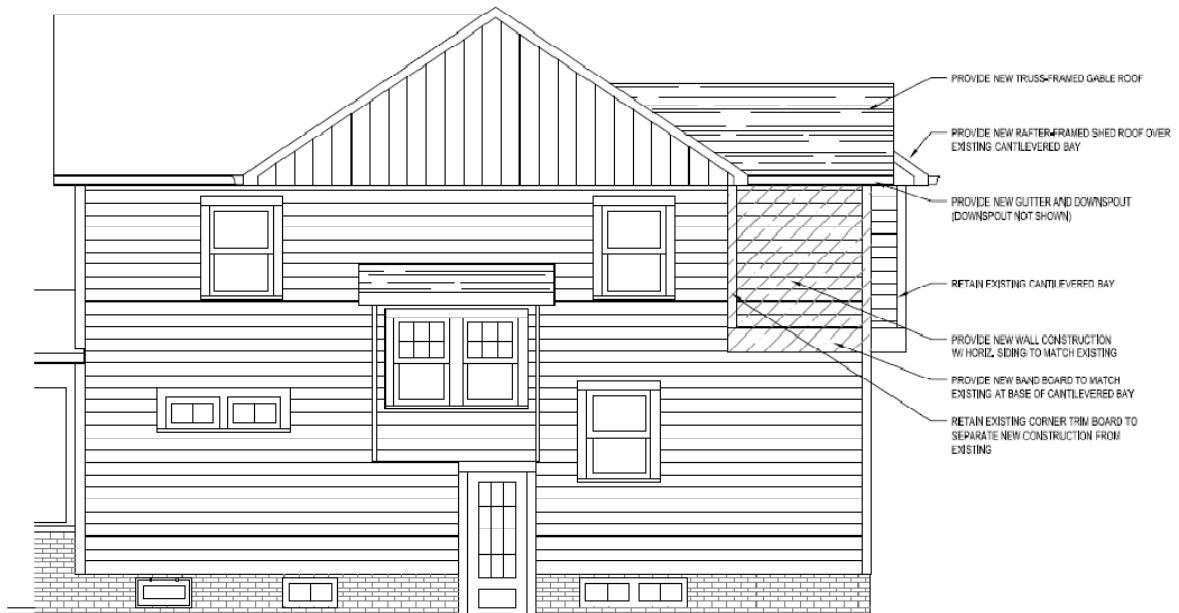
PROPOSED NORTH (SIDE) ELEVATION / SOUTH (SIDE) ELEVATION SIMILAR BUT OPPOSITE SHT. A2
